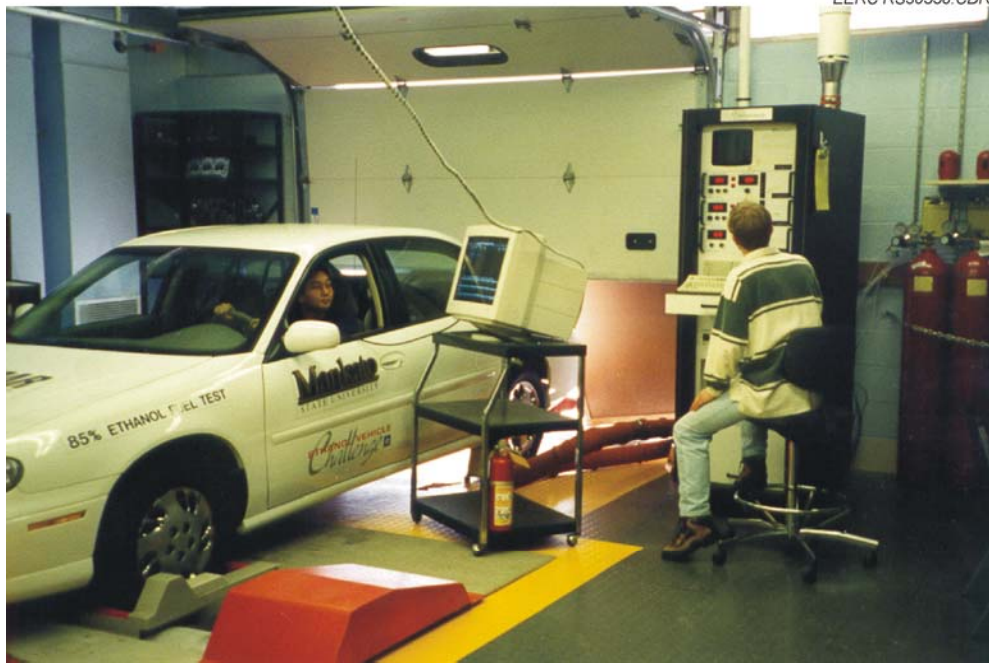
Figure 6. SuperFlow AC motor-driven chassis dynamometer.
