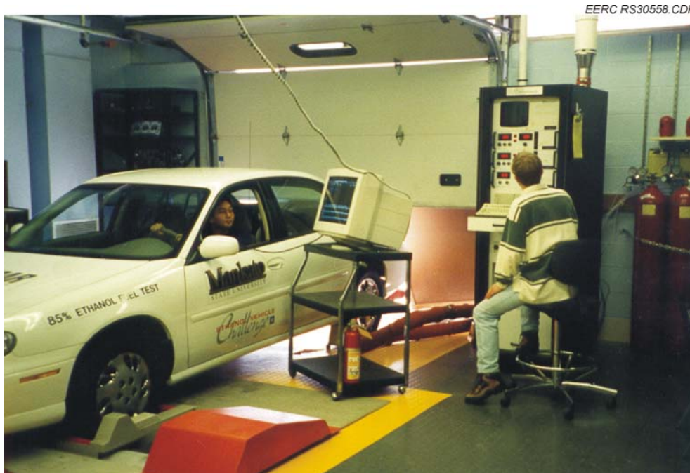
Figure 6. SuperFlow AC motor-driven chassis dynamometer.
